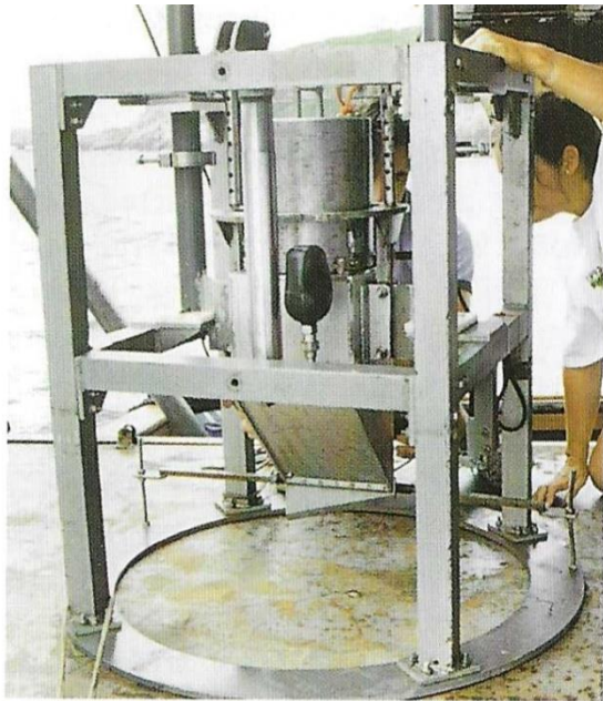
Plate 13.2 - The REMOTS system and photographs: a. REMOTS seabed camera b. a muddy seabed c. the abandoned disposal ground in Mirs Bay (大鵬灣)
